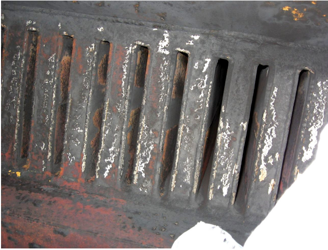
Photo 7: Tube entry DHACI rating 3
