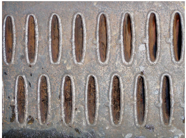
Photo 5: Tube entry DHACI rating 1
