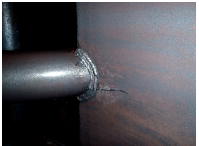
Photo 18: Crack in lower duct turning vane extending from support weld
