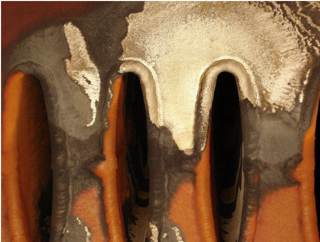
Photo 8: Tube entry DHACI rating 4
